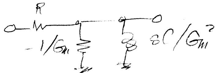
$$\frac{V_o}{V_{in}} = \frac{-R \cdot R^2 sC}{-R + R^2 sC} = \frac{-R^3 sC}{R - R^3 sC / (-R + R^2 sC)} = \frac{-R^3 sC}{-R^2} = R sC$$
